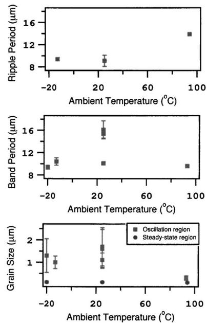
FIG. 4. Surface ripple period, microstructure (band) period, and grain size as a function of ambient temperature. The grain size refers to the single-grained darker phase.
