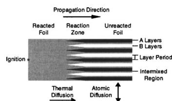
FIG. 1. A schematic of a self-propagating reaction in a binary reactive foil with the constituents (A,B) and foil parameters labeled.
