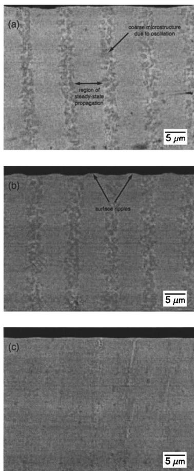
FIG. 3. SEM micrographs of Zr–Al–Cu–Ni multilayer foils reacted at (a)  $25 \text{ }^\circ\text{C}$ , (b)  $-20 \text{ }^\circ\text{C}$ , and (c)  $93 \text{ }^\circ\text{C}$ . Similar microstructural features are clearly seen in all three conditions. The reaction propagation direction is from the left-hand side to right for all samples.
