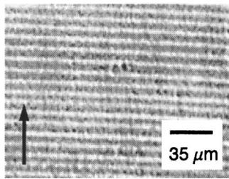
FIG. 2. Optical micrograph showing the periodic, concentric ripples that develop on the surface of a reacted foil. The arrow indicates the reaction propagation direction.
